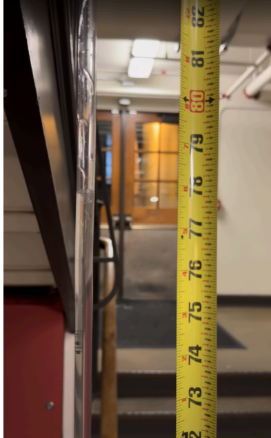
Figure 15: Water column test measurement
